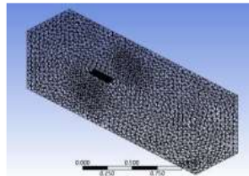
Figure 3. Meshing of test object with 6-row inline dimple formation
