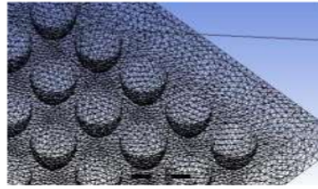
Figure 4. Detail of Meshing of the dimpled plate
